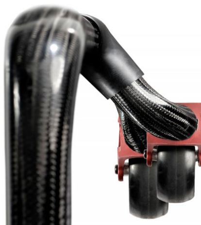
Castor house position wide vs. narrow
